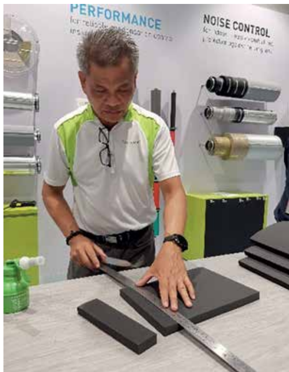
Armacell trainer, Mr Ric Matanguihan demonstrating the correct way to cut ArmaFlex insulation material.
